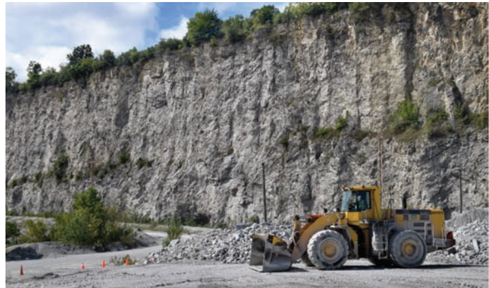
FIGURE P.6 Workers excavate limestone in a quarry near Chicago. This rock commonly consists of shells and shell fragments, and can be used in the production of concrete.
